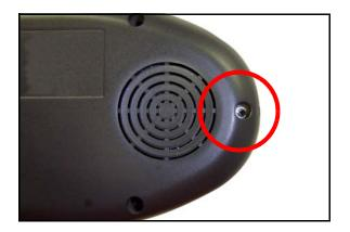
Remove the battery compartment cover.
