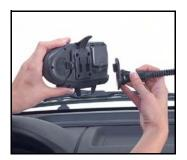
Press the windshield mount to the glass and slide the locking lever toward the glass.
