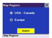
Select **Yes**. After the unit has powered down, turn the unit back on and the new map will begin loading. When it has finished, you will have access to the European maps.
